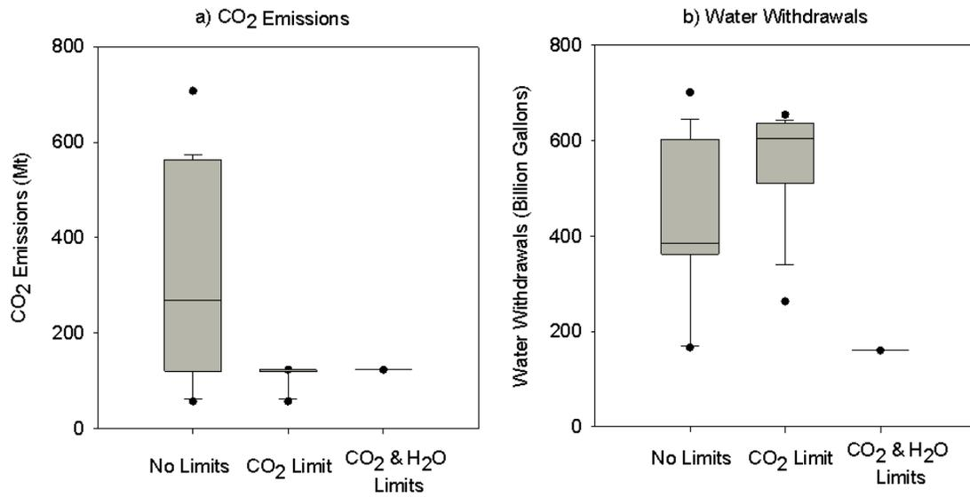
Figure 2: Uncertainty in the annual carbon dioxide emissions and water withdrawals as a function of water and carbon limits.
