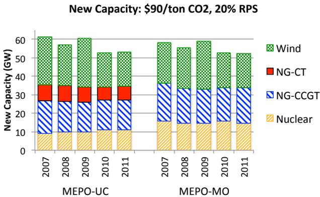
Fig. 4. Variation in optimal new capacity between 2007 baseline and alternate wind and load data years. Changing capacity wind capacity factors drives variations in total wind investment; however, the underlying flexibility differences between the MEPO-UC and MEPO-MO models remain unchanged. No new capacity was built for Coal, Coal with CCS, or NG-CCGT with CCS.
