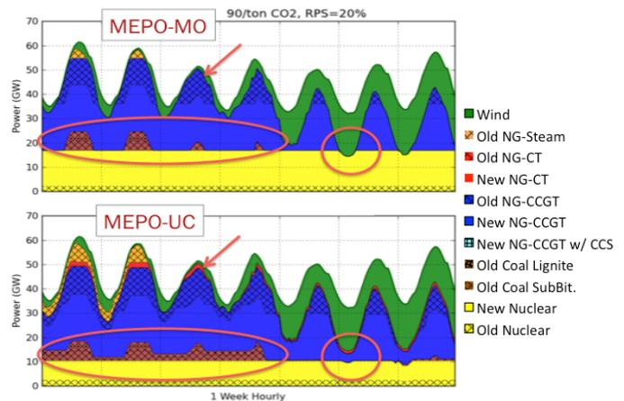
Fig. 2. Operations comparison for the week beginning August 14 as predicted using merit-order-based operations during planning (MEPO-MO, top) versus unit-commitment-based operations (MEPO-UC, bottom)
