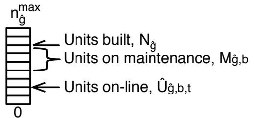
Fig. 1. Conceptual diagram of clustered capacity planning with integrated unit commitment and maintenance for a single type of unit at a single time.
