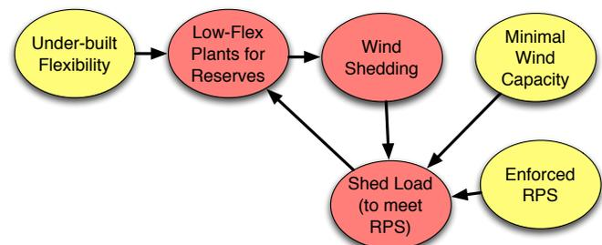
Fig. 3. Schematic description of the feedback loop that would lead to wind-shedding and load-shedding if an RPS was strictly enforced when flexibility is inadequate.
